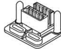
10-Position Header Housing (Accepts AMP-LEAF Crimp Snap-In and Solder Dip Contacts)
